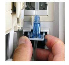
**6.** Press the tubing into the Air-in-Line Sensor located just below the Flo-Stop® fitment.
