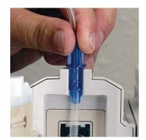
4. Position the Flo-Stop® fitment near the recess in the Medley™ Pump Module. Ensure the tubing is not twisted.
