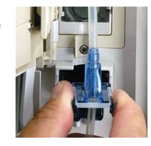
5. Press the Flo-Stop® fitment into the recess in the Medley™ Pump Module.
